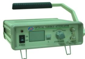
Benchtop digital variable optical attenuator support continuous optical attenuation up to 60dB at the calibration wavelengths of 850/ 1310/ 1550nm, with LCD display. The attenuation level is hold when it is turned off. With a optional rechargeable battery, it could be adopted for field applications as well as laboratory applications.
